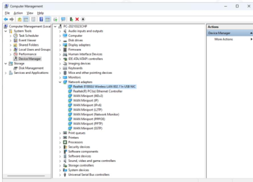
2-7 Double-click to view the device details, if there is no abnormality, the following figure shows that the driver is running normally and can view the driver details and you can view the driver details;
