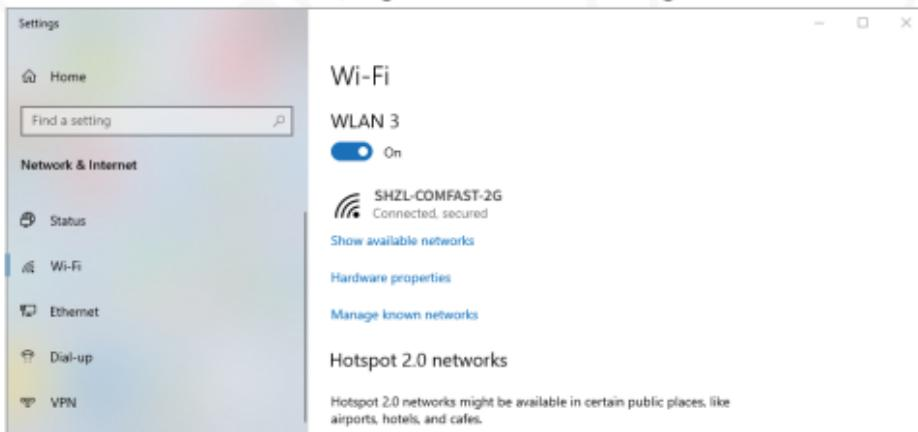
4-2 Click the "Wi-Fi" option, and then click Show connected wireless, you can view the current IP, MAC address, gateway, driver version, etc. of the wireless.
