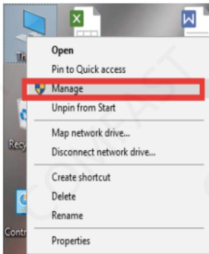
2-6 After entering the management page, click Device Manager, Network Adapter in turn, you can see the installed network card driver;
