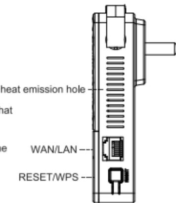
**WPS/Reset:** Press the less than 5 seconds to use WPS auto pairing; Long press for more than 5 seconds to reset to factory settings.
