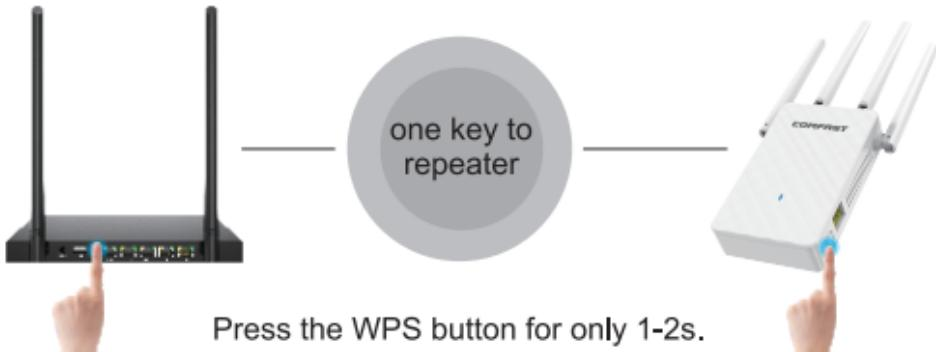
Please make sure that the device was not connected with other routers' network before using WPS. If connected, press the RESET button to restore factory settings and then start to use WPS.
