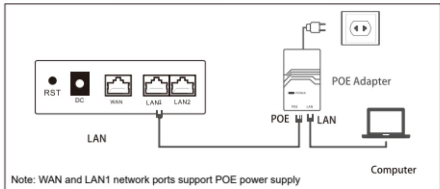
2. Set the computer to obtain the IP address automatically, and connect the LAN1 port of the device to the device management interface.
