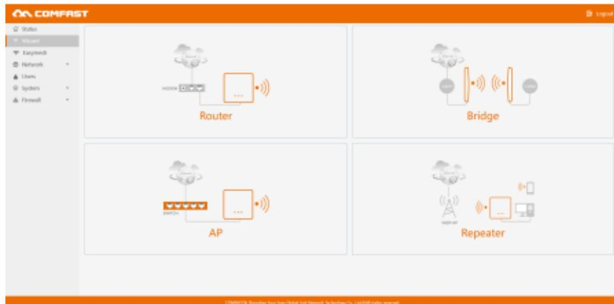
5. Click AP mode and set up IP Address and Subnet Mask. The IP address and Subnet mask should be within the same network segment as upper network and can't be conflict with IP address from upper network router. After settings, you can visit the device from the IP address you have set just now by connecting internet with WAN port of the device or POE adapter LAN port.
