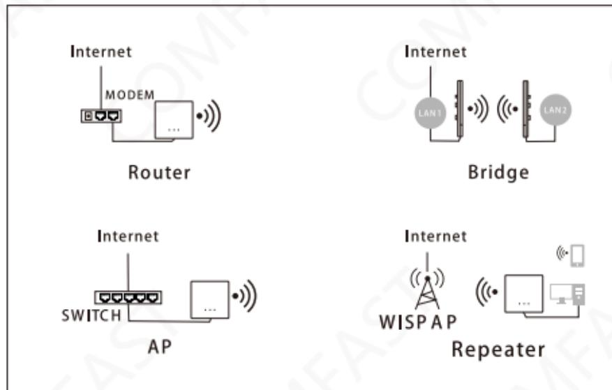
5. Click AP mode and set up IP Address and Subnet Mask. The IP address and Subnet mask should be within the same network segment as upper network and can't be conflict with IP address from upper network router. After settings, you can visit the device from the IP address you have set just now by connecting internet with WAN port of the device or POE adapter LAN port.
