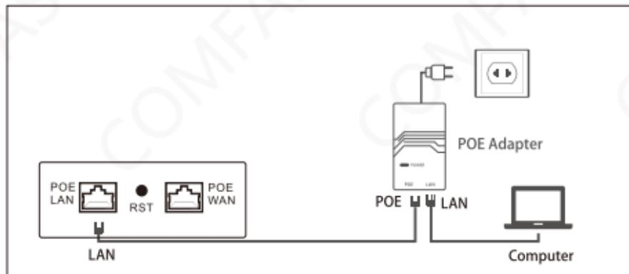
2. Set the computer to obtain the IP address automatically, and connect the LAN port of the device to the device management interface.
