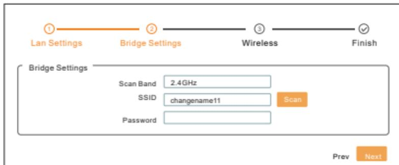
(3) Set the SSID name and password of the 2.4G of the AP.
