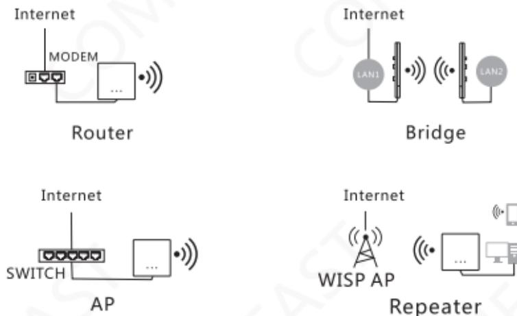
5. Click AP mode and set up IP Address and Subnet Mask. The IP address and Subnet mask should be within the same network segment as upper network and can't be conflict with IP address from upper network router. After settings, you can visit the device from the IP address you have set just now by connecting internet with WAN port of the device or POE adapter LAN port.
