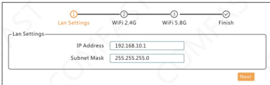
6. AP Mode: You can set up 2.4G/5.8G wireless SSID, password, channel and country in advance. After setting up, the device's WAN port or POE adapter LAN port connected internet, other mobile devices can connect the SSID to surf the internet.
