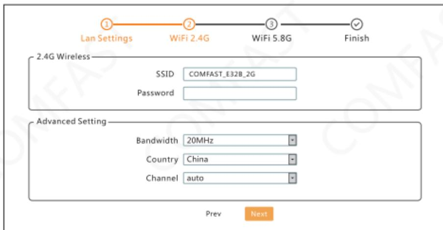
7. Bridge Mode: Pls ensure the WDS in upper network is enabled. AP device can set up intranet segment(do not set the same IP address as the upper router), and then select the wireless SSID signal you need to bridge(Distinguish between 5.8GHz and 2.4GHz) and input wireless password.
