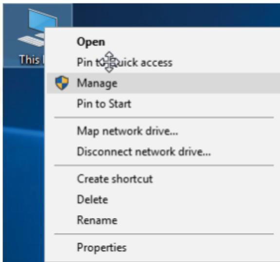
2-5 After entering the management page, click Device Manager, Network Adapter in turn, you can see the installed network card driver (Note: This step requires the network card to be connected to the computer to see it.)
