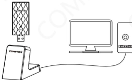
Note: When using a desktop computer, it is recommended to use a USB extension cord base to connect to the port on the back of the computer case (some desktop ports have insufficient power supply or cannot be used), and extend it to the Desktop computer usb ports.
